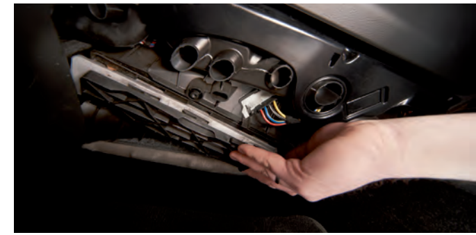
Remove the pollen filter to expose the evaporator according to the vehicle manufacturer's instructions.
