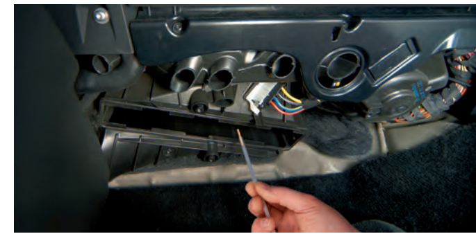
Insert the hose with rotor nozzle into the evaporator.
