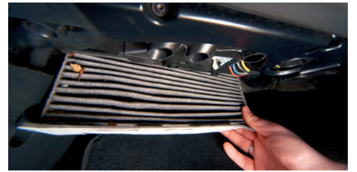
Disassemble the pollen filter.
